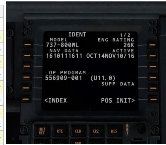
Modern FMS installed on a 737-800WL
